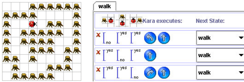
Fig. 2.1: Finite state machine to control circuit walk of ladybug
