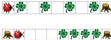
Fig. 3.13: Top: A pattern recognizable by a state machine (i.e., (01)^n ). Bottom: A pattern not recognizable by a state machine (i.e., 0^n 1^n ).
