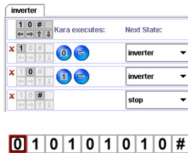
Fig. 4.6: The inverter Turing machine to be simulated
